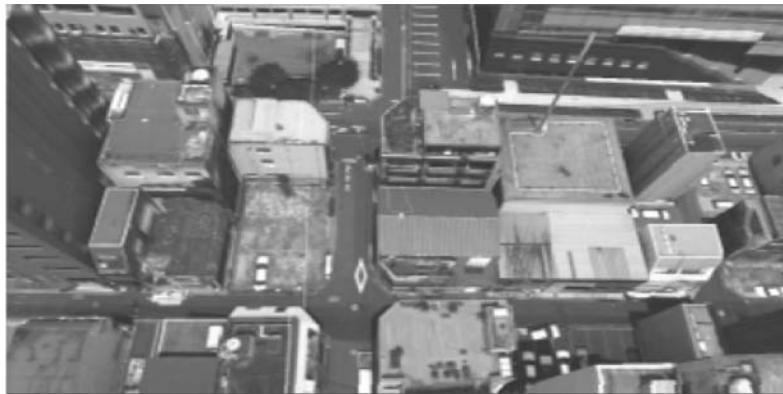
Fig.2.14. 3-D reference data (precise 3-D data) constructed from three-line sensor images
