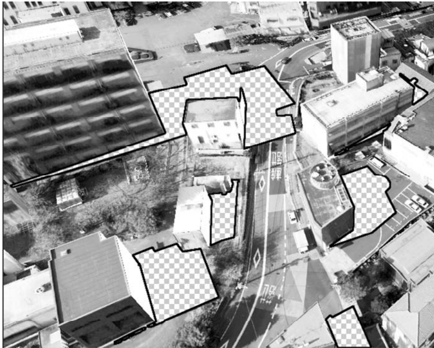
Fig.2.11. Detection of shadow area using the geometrical approach
